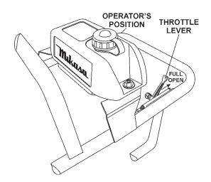
Figure 12. Throttle Lever (Full Open)
